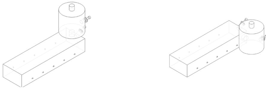
(a) Secondary chamber located above the primary chamber (Model C1)
